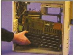
The busboard then fits on to the connector. Three screws hold it in place – plus, two support it at the rear. It all fits in pretty easily, with no real brute force required.
