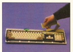
First, you have to get the A1200 motherboard out. This involves unscrewing the case, unplugging the floppy drive, keyboard and removing the metal screening.
